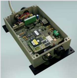
Tractor-based Operating Electronics for the YARA N-Sensor, including processing electronics and spectral sensors in IP65 housing.
