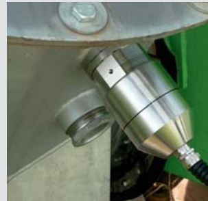
NIRON reflection head with integrated light source and internal white reference
