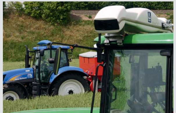
Tractor-based Operating Electronics for the YARA N-Sensor, including processing electronics and Spectral Sensors in IP65 housing.
