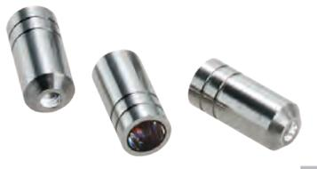
Rods and cylinders are formed from thick fibers with diameters greater than 1 mm. Rods of almost any diameter can be created and used as functional parts such as homogenizers. Since the thickness reduces the fragility of thinner fibers, the heat-sensitive coating is no longer required, and the fiber-optic element can direct light into extreme environments. The diameter of a rod can be customized.
