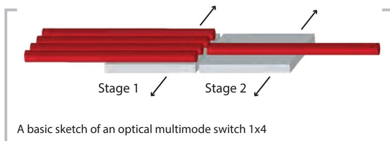
The elements are made from high-precision ceramic parts to achieve high accuracy and reproducibility. These parts are moved by piezo-electric elements to guarantee fast and reliable positioning.
