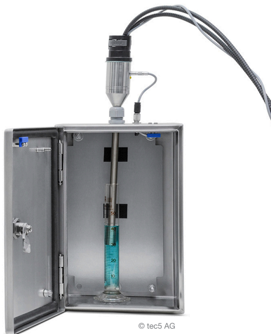
[ Raman installation for measurements in a probe chamber ]
