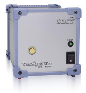
High performance spectrometer system with Ethernet interface and integrated data preprocessing. Equipped with a wide-range Spectral Sensor, the unit is ideal for use in laboratories or Ethernet networks. An F-SMA fiber connector as optical input allows easy connection of fiber-based probes or measurement assemblies.
