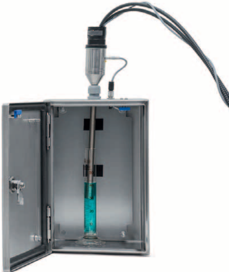
[ Figure 4: Example of a Raman installation for a measurement in a probe chamber. The Raman probe head is connected with a measurement box. During measurement the external interlock [external-IL1] ensures a permanent connection of the probe head. The probe head cannot be unmounted from the box without disconnecting the interlock-cable. An interlock-switch at the door of the box [blue] which is connected in serial to the external-IL1 further ensures the laser can be switched-on only when the door is closed. If the interlock-loop is opened, the laser will be switched-off automatically. ]
